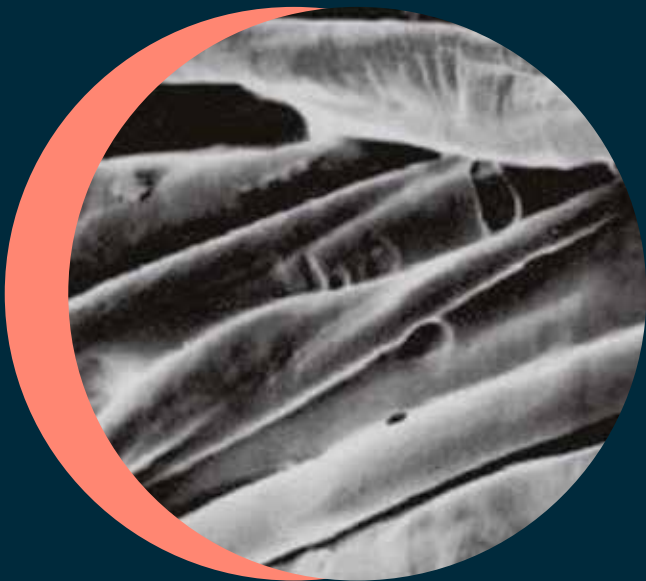
Elvanol™ T-25 polyvinyl alcohol (570X)
