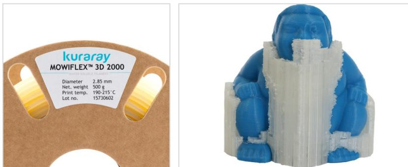
**[Photos 3 and 4] Support structures that can be washed away: the PVOH-based polymer blend MOWIFLEX™ 3D 2000 is Kuraray's first product for 3D printing. This filament can be used to produce support structures for demanding shapes and simply dissolved in water after printing.**
