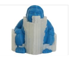
[Photos 3 and 4] Support structures that can be washed away: the PVOH-based polymer blend MOWIFLEX™ 3D 2000 is Kuraray's first product for 3D printing. This filament can be used to produce support structures for demanding shapes and simply dissolved in water after printing.
