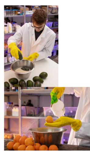
**[Photos 4 and 5]** An environmentally compatible protective coating: a very thin layer of Liquidseal coating is applied directly to the peel of oranges, lemons, mangoes and avocados. Liquidseal has very good environmental compatibility and is 100 percent biodegradable and compostable. Kuraray's PVOH materials play a key role in this. (Photos: Liquidseal)
